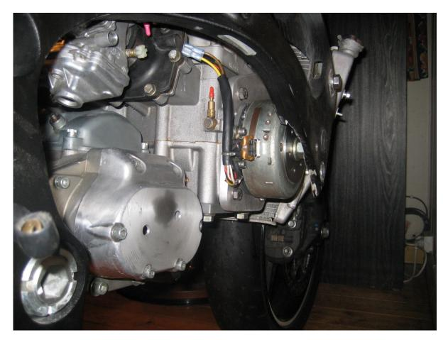
With the FXR transmission in house, I started to work on how I could assemble the engine to the gearbox. The Polaris engine has only 4 holes with threads on the bottom of the engine case. In a sled,
