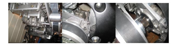
Well, the tranny and engine had to be assembled some way, so I started cutting off excessive material to make the tranny shorter. I made a flange at the rear where I installed threads for bolting a bracket. The bracket would function as the rear engine mounts. On the front end of the tranny, there where two attachment bolts. I made a stiff aluminium plate under the engine case which connected engine and tranny.
